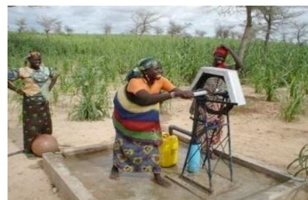
Rope pump in use in Dasga Haoussa
